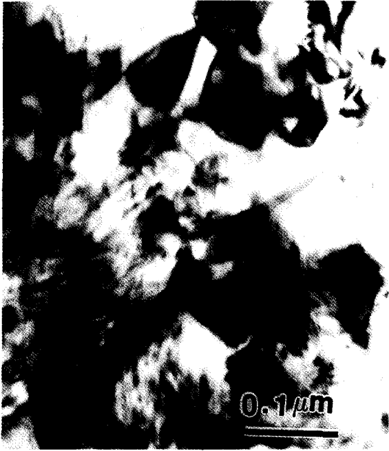
Fig. 15. TEM of specimen D (shear displacement of 0.46 mm); equiaxed micro-grains.
